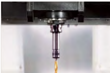
Through-spindle coolant system
