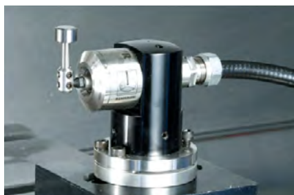
Auto tool measurement device
