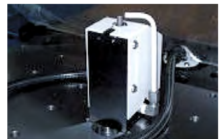
Auto tool measurement device
